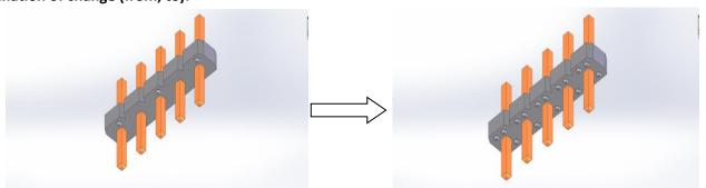
Reason for change: Improvement on the 1 & 2 positions (cut) header sit flat on the PCB.
